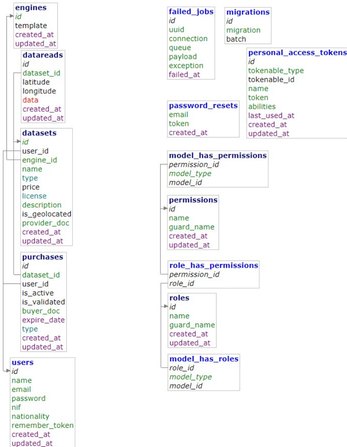
Figure 20: Database structure for the Agriculture dataspace.
